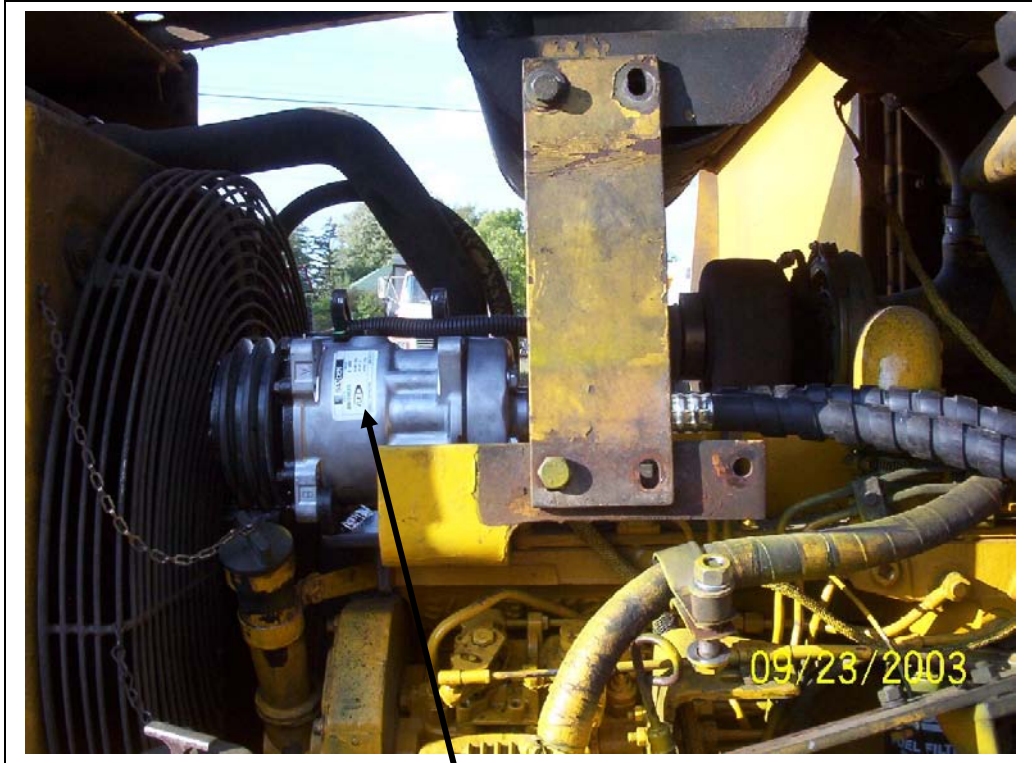
Compressor in place without 2 inch spacer
