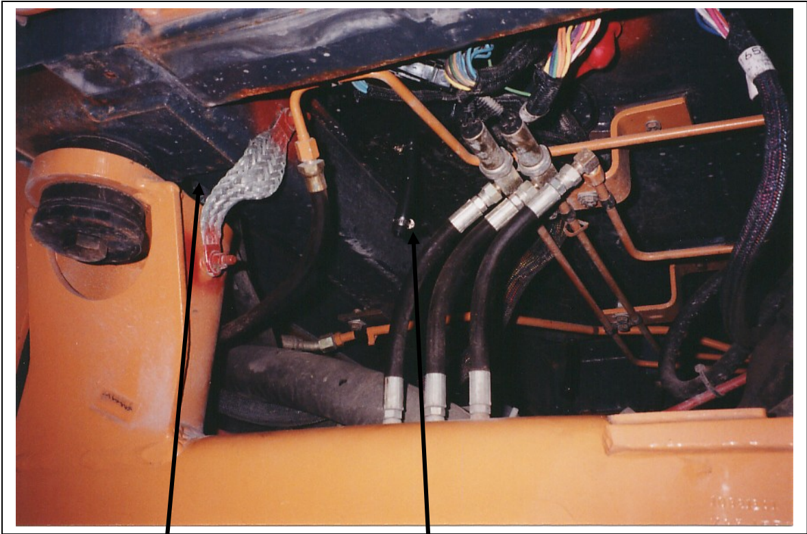
A/C hoses entering the cab
