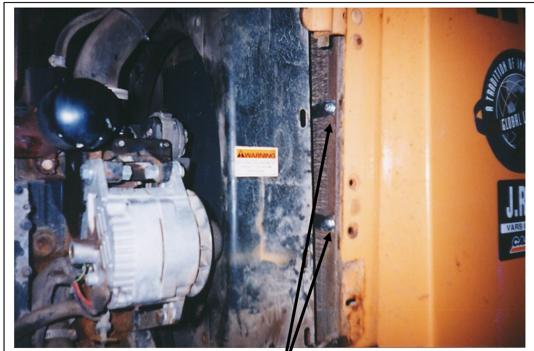
Condenser brackets on left side of radiator
